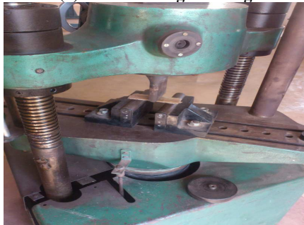
(c) Flexural strength testing Figure 5: Composite Testing
