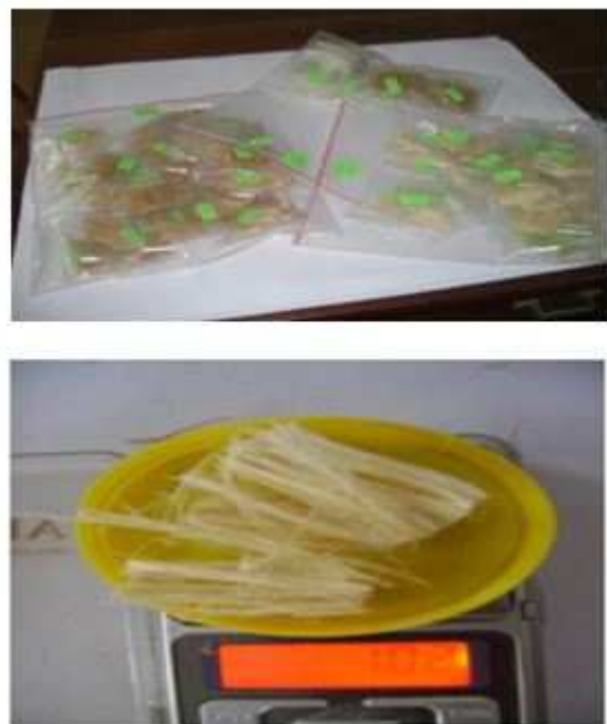
Figure 1: Fibers after chemical treatment
